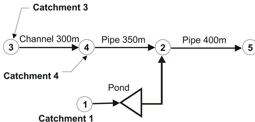
In this tutorial we will use the **Next Link** option because we want to add the runoff from area 4 and design a 350m pipe to carry the total flow to the junction at node 2.
