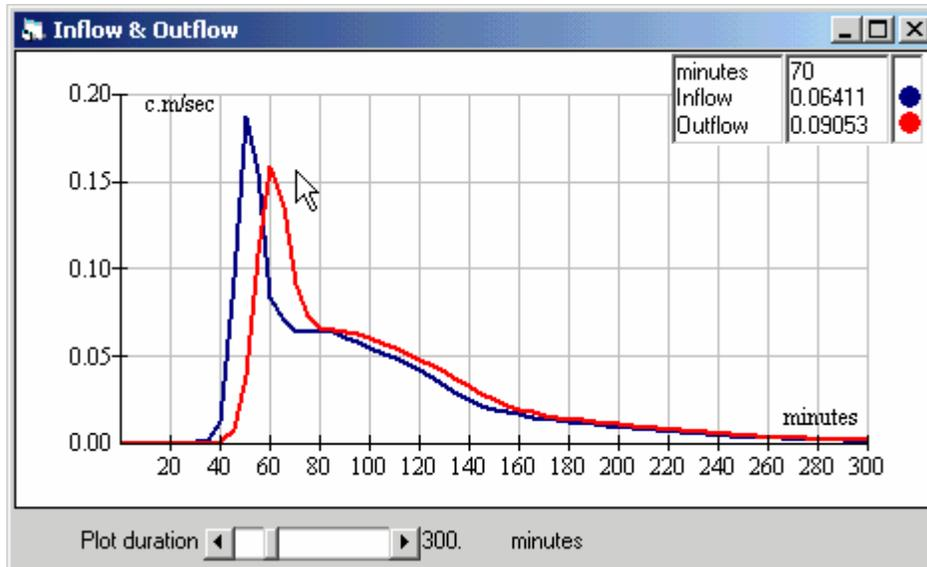
Note the peak is reduced from 0.188 c.m/s to 0.158 c.m/s and lagged by about 10 minutes. Since the hydrographs are plotted at 5 minute increments, very 'peaky' hydrographs may sometimes show some truncation of the outflow.
