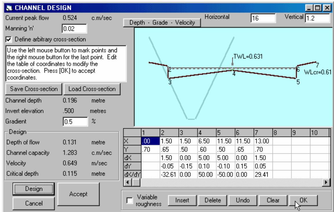
You have the option at this point of saving the cross section to a file which can be reused in future design sessions. In this instance we do not need to do this because MIDUSS remembers this particular cross section from this point forward in the design session.
