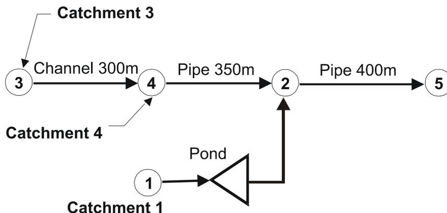
The above diagram shows a network comprising 5 nodes and 4 links. Because only one outflow link exists for each node the link number is the same as the upstream node.
