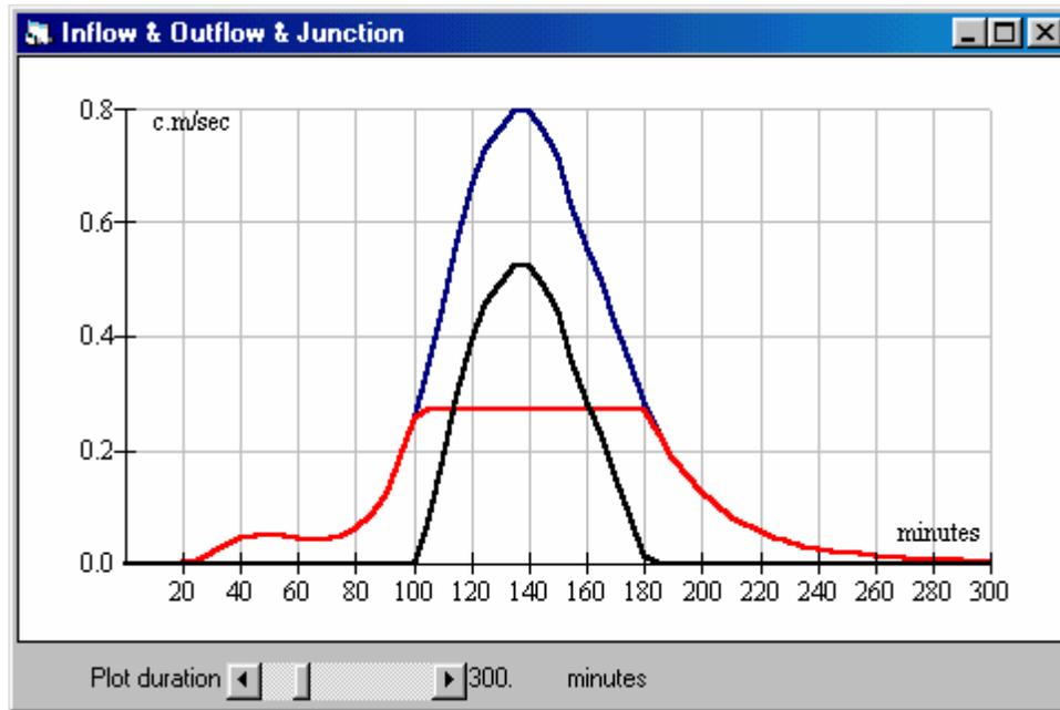
The outflow from the diversion can now be converted to the inflow to the pipe by using the Hydrograph / Next Link command. If the Diversion command was invoked by a surcharged pipe, MIDUSS will do this automatically so all you need to do is acknowledge this action.
