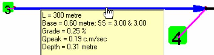
Note that MIDUSS scales the layout conduits after you have used the Route command. However, you can move the elements around and shrink them or enlarge them as you see fit. The actual design length used in the MIDUSS session is not changed – only the visual interpretation on the layout.
