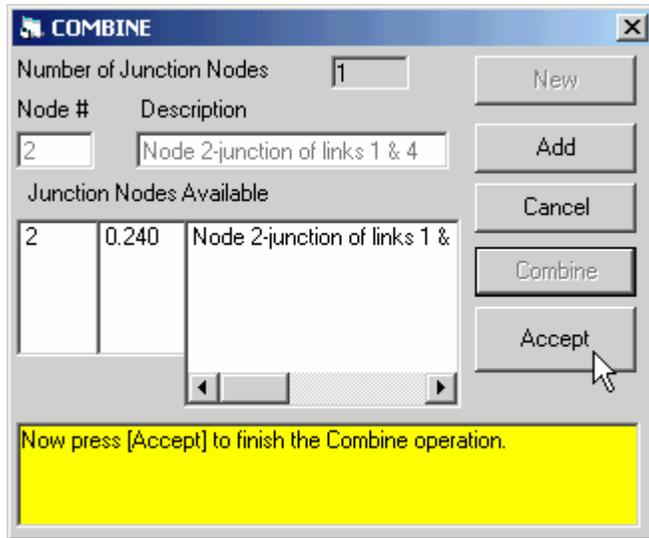
The Combine form is closed and the Peak Flows table is updated with another record showing the Combine operation, the node number and the updated peak flow of the Junction hydrograph as shown below. Note that in the illustration below, the height of the Peak Flows table has been increased by dragging the top edge of the window upwards.
