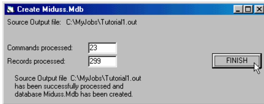
This is where the input file is processed into a file named MIDUSS.Mdb. This is a quasi-database file that MIDUSS uses to process all the commands and data in an organized manner.
