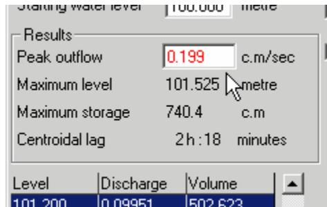
From the Pond Design form it is clear that the design is conservative. The peak outflow is only 0.199 c.m/s – well below the target outflow of 0.3 c.m/s and the storage volume is too large at 740.4 c.m. The weir is overtopped by a head of 125mm (101.525 – 101.400) for about 55 minutes.
