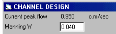
Figure 4-12 – Setting the Manning ‘n’ value for the channel
